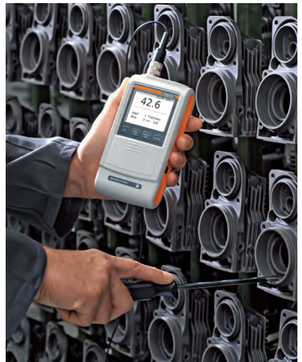
Measurements using the internal probe FAI 3.3-150
