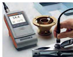
DUALSCOPE® FMP40 using probe FD13H
